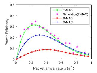
Figure 8. The power efficiency for T-MAC, S-MAC and X-MAC protocols versus packet arrival rate.
