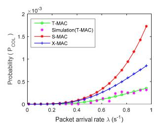
**Figure 3.** The collision probability  $P_{COL}$  in a cycle versus the packet arrival rate  $\times$  for the T-MAC, S-MAC and X-MAC protocols.
