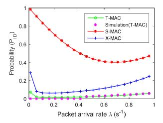
**Figure 2.** The idle probability  $P_{ID}$  in a cycle versus the packet arrival rate  $\times$  for the T-MAC, S-MAC and X-MAC protocols.
