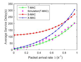
**Figure 5.** The average service delay with respect to the packet arrival rate  $\times$  for the T-MAC, S-MAC and X-MAC protocols.
