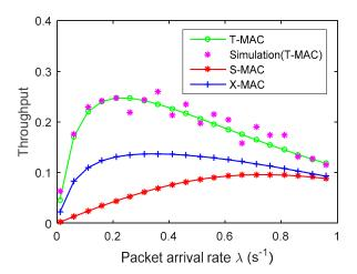
**Figure 6.** The throughput versus packet arrival rate  $\times$  for the T-MAC, S-MAC and X-MAC protocols.
