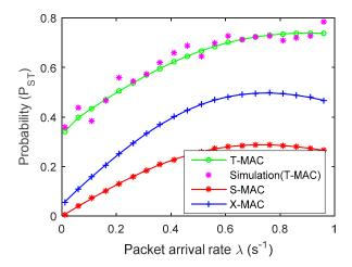
**Figure 4.** The successful transmission probability,  $P_{ST}$ , in a cycle versus different packet arrival rates  $\lambda$ , for the T-MAC, S-MAC and X-MAC protocols.
