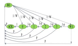
Figure 1. Discrete time Markov Chain of T-MAC Protocol.
